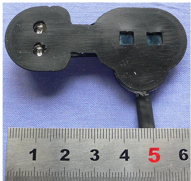
Figure 8 The new probe of the TSAH-100 NIRS with two different distances (30 mm and 40 mm). Left: light source; Right: detectors.
