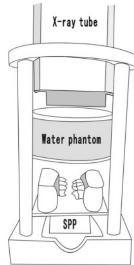
Figure 1 Schematic of the geometry for exposing test radiographs. SPP, storage phosphor plate
