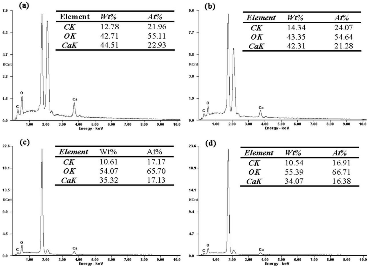
FIGURE 3. EDS spectra of microcapsules: (a) Formula A, (b) Formula B, (c) Formula C, (d) Formula D.
