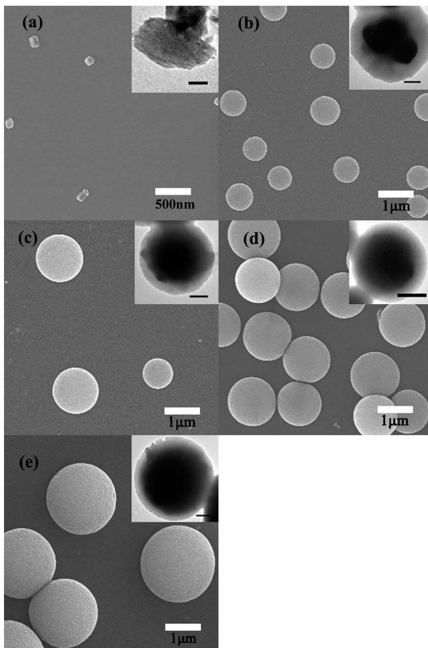
**FIGURE 1.** SEM and TEM (inset figure) images of microcapsules: (a) Pure calcium hydroxide (the bar in the inset figure represents 50 nm), (b) Formula A (the bar in the inset figure represents 100 nm), (c) Formula B (the bar in the inset figure represents 200 nm), (d) Formula C (the bar in the inset figure represents 500 nm), (e) Formula D (the bar in the inset figure represents 500 nm).
