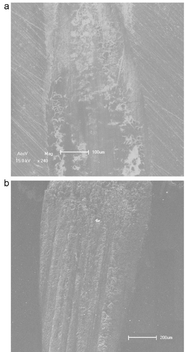
Fig. 5. SEM images of the worn surface of the natural enamel after wear test for 5400 cycles against zirconia. Small cracks and enamel flakes spreading entire wear scar were observed on the worn surface of enamel against polished zirconia (a). Deep parallel furrows were observed on the worn surface of enamel against rough zirconia (b).
