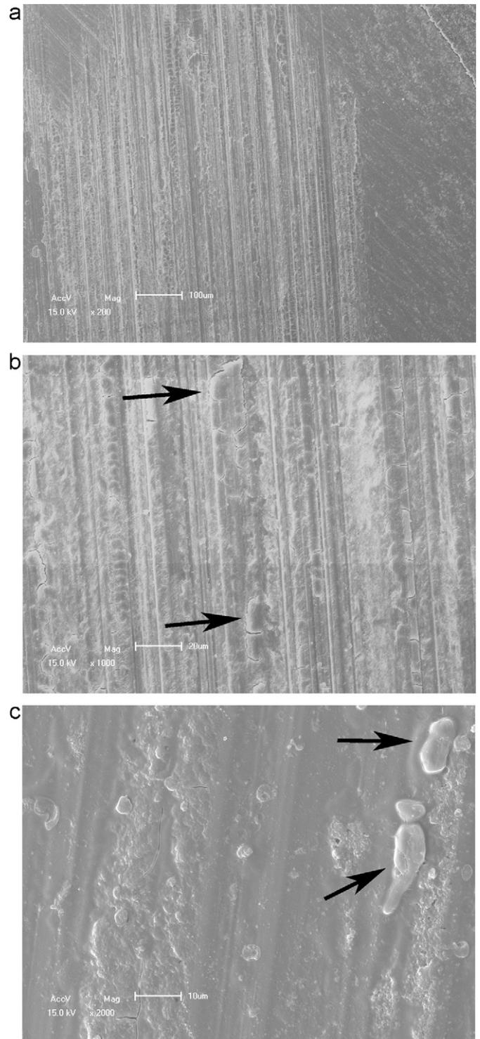
Fig. 3. SEM images of the worn surface of enamel after wear test for 5400 cycles against Empress showing the formation of rough parallel furrows (a). A high magnification image of “a” revealing the formation of small cracks (marked by arrows) within the furrows (b). The observed particles sticking on the the surface of Empress antagonist was ascribed to the accumulation of chipped off enamel and glass ceramic particles (c).
