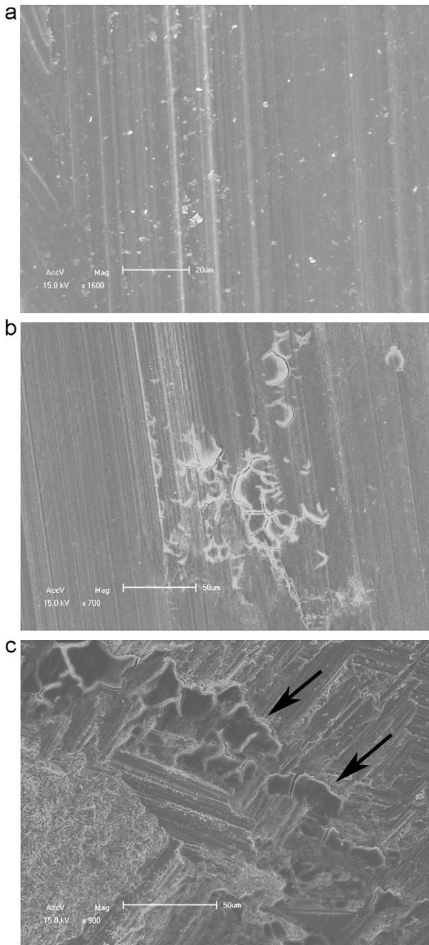
Fig. 7. High magnification SEM micrographs showing the formation of furrows with small particles (a) and small cracks (b) on the worn surface of enamel against rough zirconia. The observed small flakes (marked by arrows) on the surface of antagonist zirconia was ascribed to the accumulation of enamel chipped off (c).
