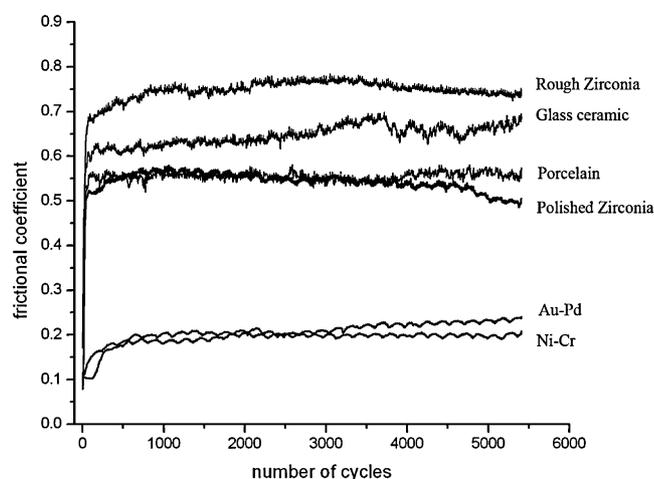
Fig. 1. The frictional coefficient of natural enamel against different dental materials plotted versus the number of cycles.
