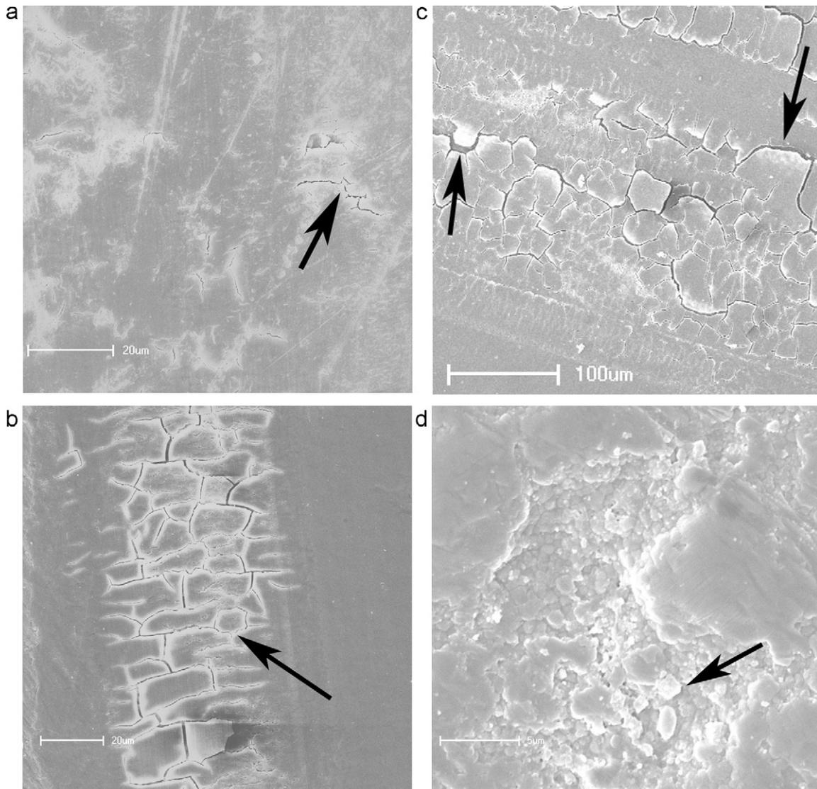
Fig. 6. High magnification SEM micrographs showing the typical damages of enamel against polished zirconia: small cracks (a, marked by arrow), reticular cracks (b) and chipping flakes (c, marked by arrow). The surface damage of zirconia was classified as grains peeling-off (d, marked by arrow).
