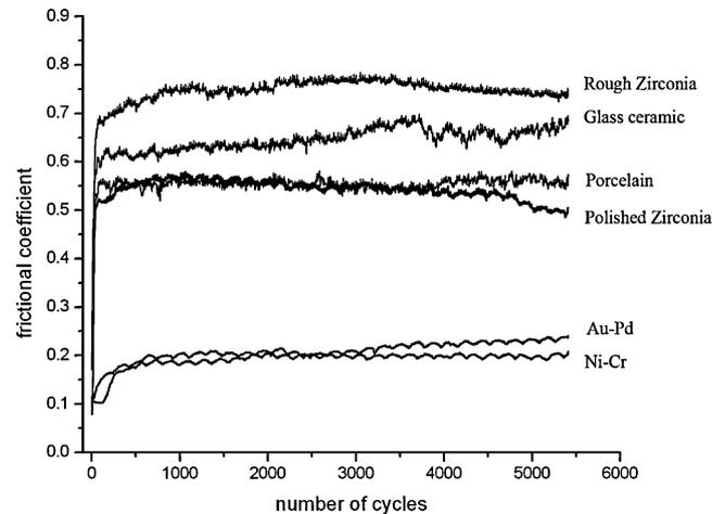
Fig. 1. The frictional coefficient of natural enamel against different dental materials plotted versus the number of cycles.
