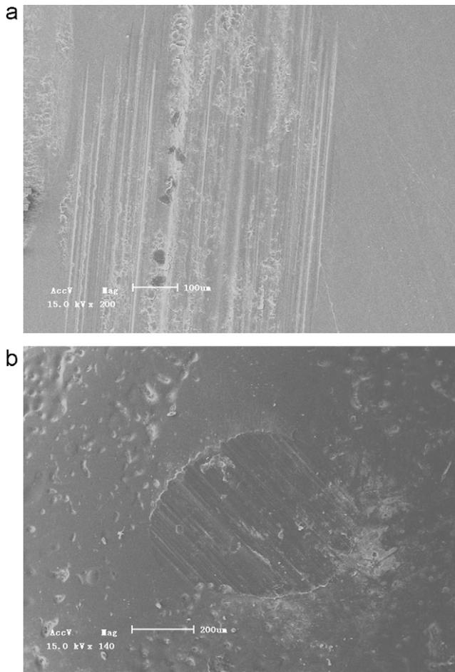
Fig. 4. SEM micrograph of the worn surface of enamel after wear test for 5400 cycles against porcelain showing the formation of parallel furrows (a). Similar parallel furrows were also observed on the surface of porcelain antagonist (b).
