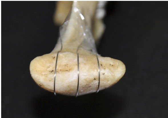
Fig. 1. Orthodontic ligature wires were wrapped over the condylar head and neck surface within planes perpendicular to the horizontal axis of the condyle.
