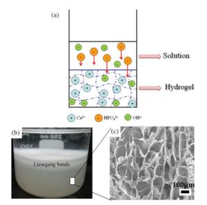
Figure 1. (a) Schematic drawing for the mineralization of hydrogel. (b) The digital photo and (c) SEM micrograph of 3D porous hydrogel scaffold fabricated by freeze drying.
