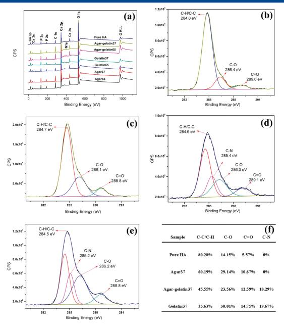
Figure 4. Surface atomic composition of as-prepared apatite under different conditions: XPS wide spectrum of all samples (a); high-resolution spectrum of carbon peaks (C1s) for pure HA (b), Agar37 (c), Agar-gelatin37 (d) and Gelatin37 (e); and the contents of relative functional groups (f).
