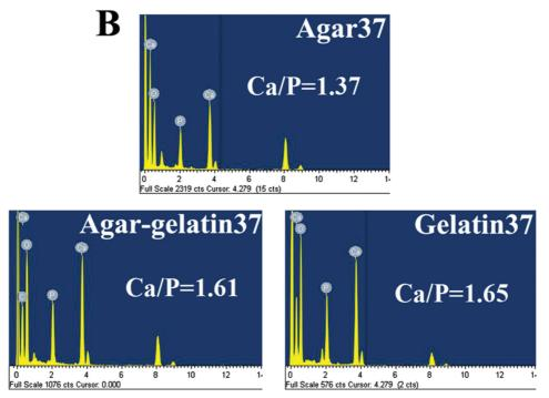
Figure 6. (A) SEM images of the agar-based hydrogels and as-prepared apatite under different conditions: (a) agar hydrogel; (b) Agar37; (c) Agar65; (d) agar-gelatin hybrid hydrogel; (e) Agar-gelatin37; (f) Agar-gelatin65; (g) Gelatin37; (h) Gelatin65 and (i) pure HA. The insets (b) and (e) show the high resolution SEM images of the corresponding apatite crystals. B is corresponding Energy Dispersive X-ray (EDX) spectroscopy.
