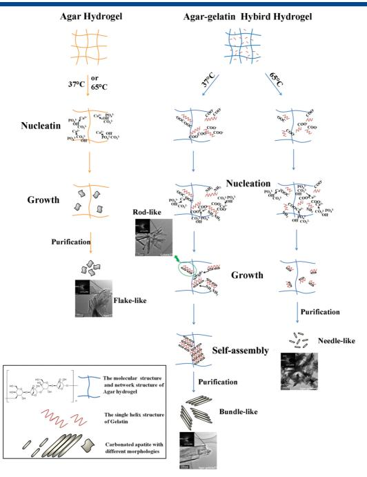
Scheme 1. Schematic drawing of the formation and self-assembling mechanism of the carbonated apatite in agar-based hydrogels.
