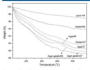
Figure 5. TGA profiles of as-prepared apatite under different conditions.
