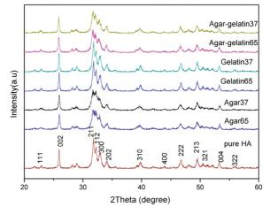
Figure 2. XRD spectra of as-prepared apatite under different conditions.
