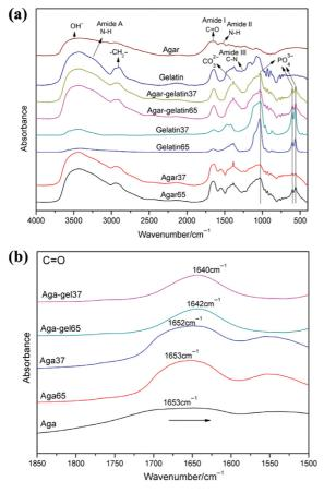
Figure 3. (a) FTIR spectra of mineralized hydrogels under different conditions; (b) a shift of C=O band in FT-IR enlarged patterns.
