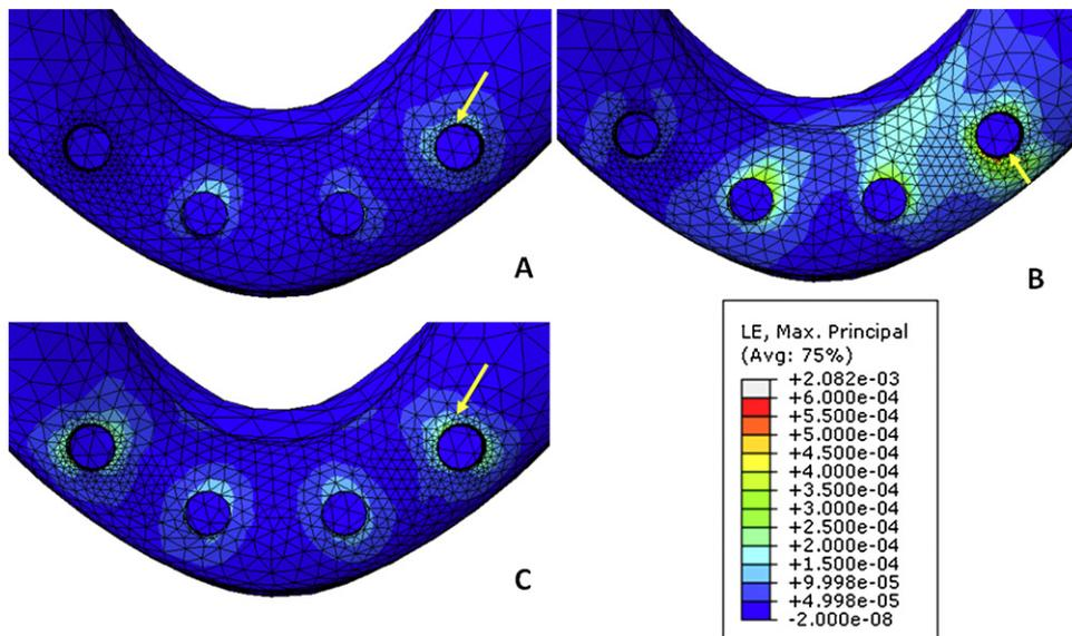
**Fig. 5 – Equivalent strain distribution in the cortical bone of model D under three loading conditions ((A) VM, (B) IM and (C) VI). Colours indicate level of strain from dark blue (lowest) to red (highest). The arrows show the sites at which peak strain values occur.**
