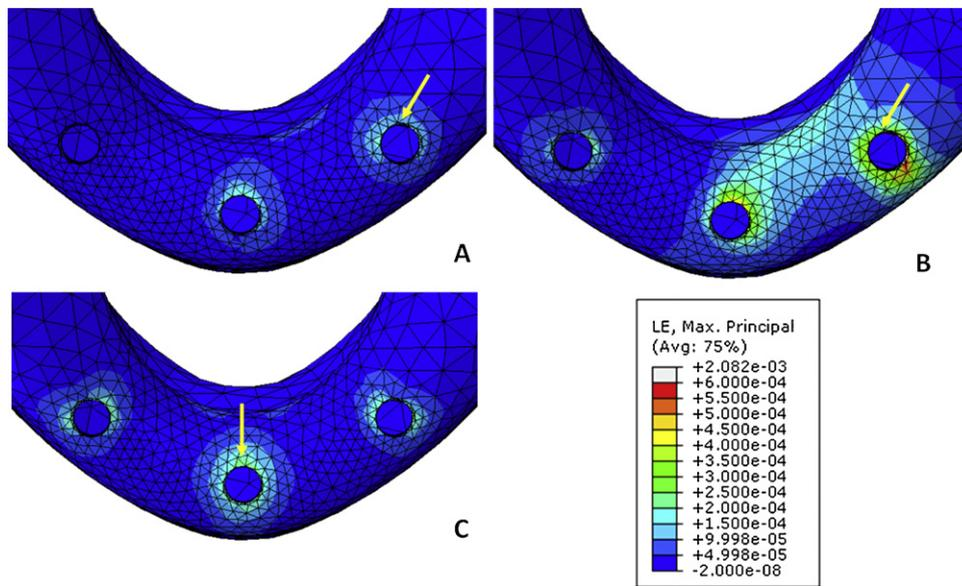
**Fig. 4 – Equivalent strain distribution in the cortical bone of model C under three loading conditions ((A) VM, (B) IM and (C) VI). Colours indicate level of strain from dark blue (lowest) to red (highest). The arrows show the sites at which peak strain values occur.**
