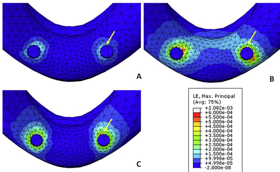
**Fig. 3 – Equivalent strain distribution in the cortical bone of model B under three loading conditions ((A) VM, (B) IM and (C) VI). Colours indicate level of strain from dark blue (lowest) to red (highest). The arrows show the sites at which peak strain values occur.**
