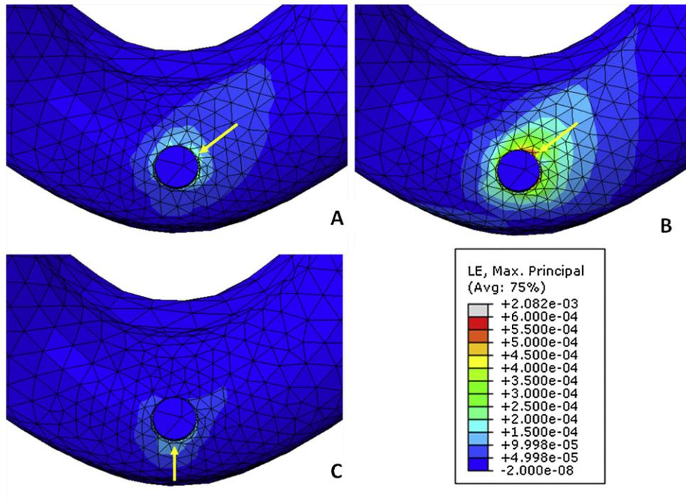
**Fig. 2 – Equivalent strain distribution in the cortical bone of model A under three loading conditions ((A) VM, (B) IM and (C) VI). Colours indicate level of strain from dark blue (lowest) to red (highest). The arrows show the sites at which peak strain values occur.**
