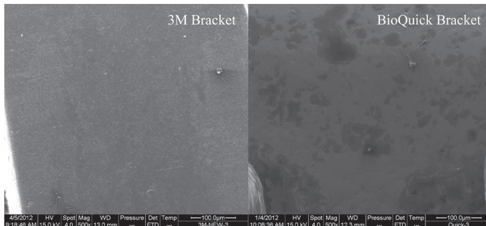
Fig 3. SEM images of the two types of stainless steel brackets. Original magnification, 500 $\times$ . The slot surface of the BioQuick bracket (right) appears more irregular than that of the 3M bracket (left) before treatment.
