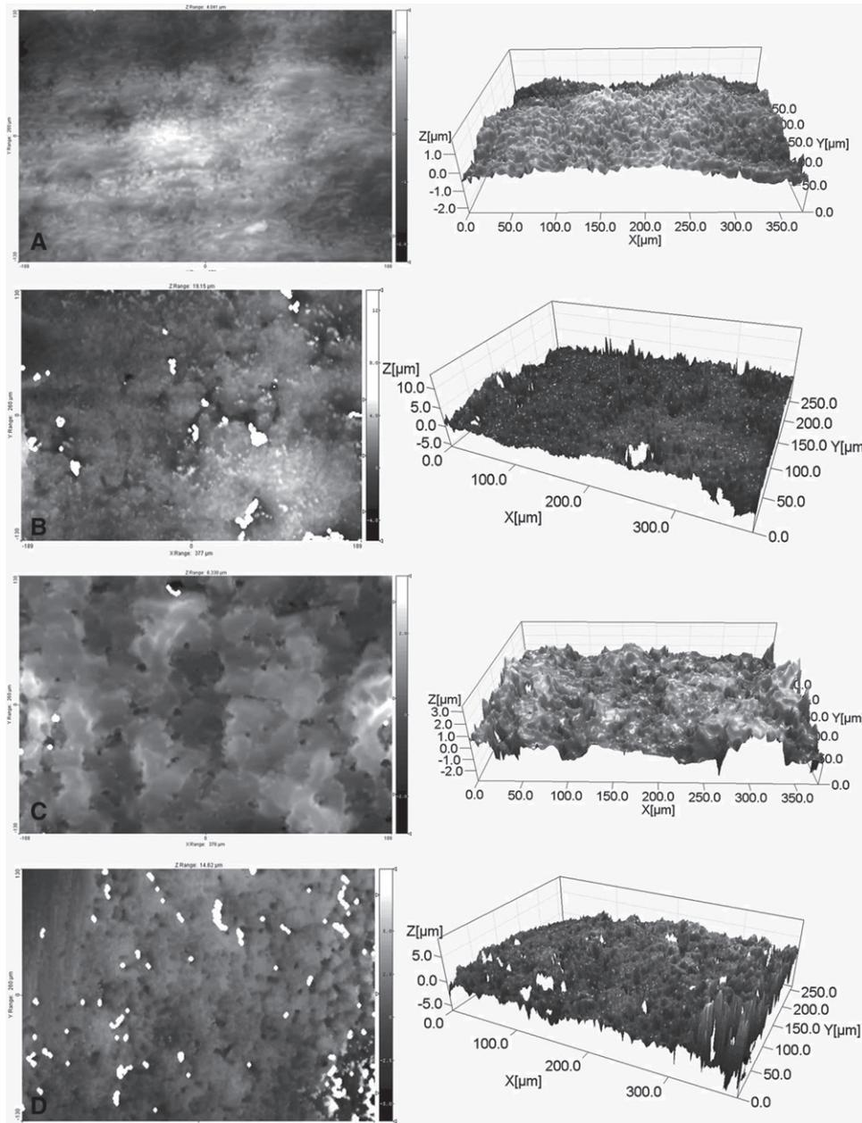
Fig 5. Representative white-light interferometry profilometer topographies and 3D images of the bracket slot surfaces: (a) 3M new bracket, (b) 3M retrieved bracket, (c) BioQuick new bracket, (d) BioQuick retrieved bracket.
