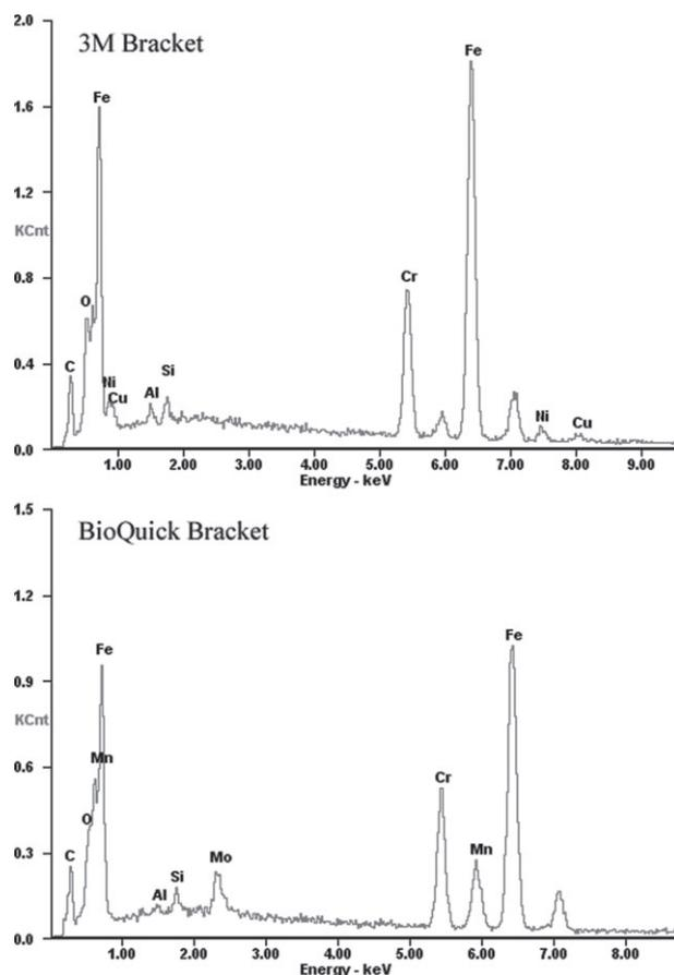
Fig 4. EDS analysis of the elemental composition of the new bracket surface slots. The main components of the two brands of brackets are identical, but the trace components differ somewhat.
