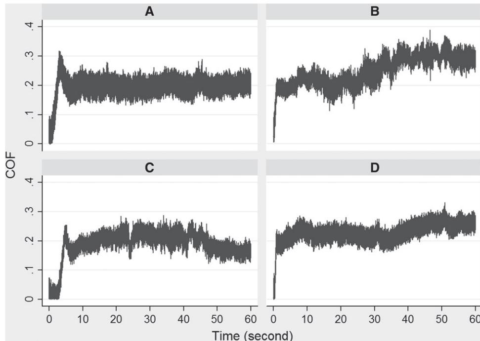
Fig 2. Representative COF findings with respect to the four groups of brackets: (a) 3M new bracket, (b) 3M retrieved bracket, (c) BioQuick new bracket, (d) BioQuick retrieved bracket. The COF was calculated by averaging that registered between the 10th and 60th s.
