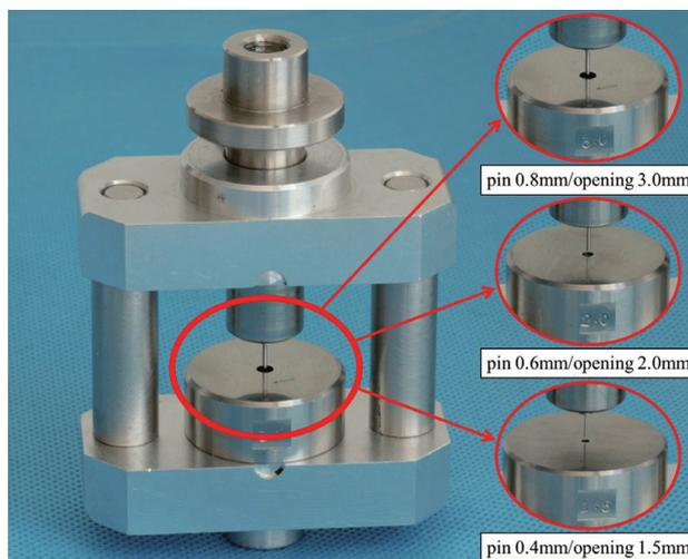
Fig. 2 The loading fixtures for thin slice push-out test.
