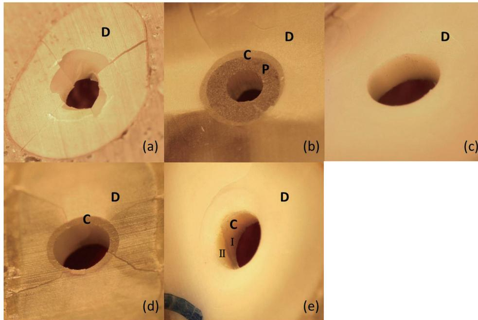
Fig. 4 The failure mode of debonded specimens.
