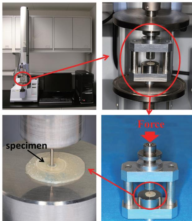
Fig. 3 The thin slice push-out test.
