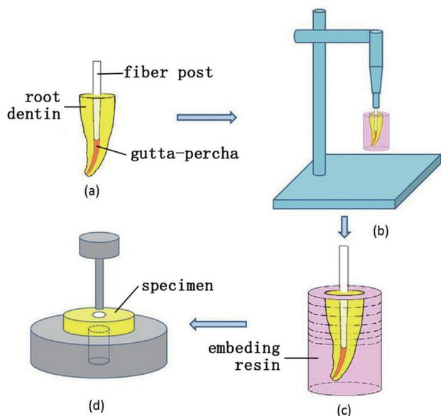
Fig. 1 Schema of the experimental procedures of the thin slice push-out test.
