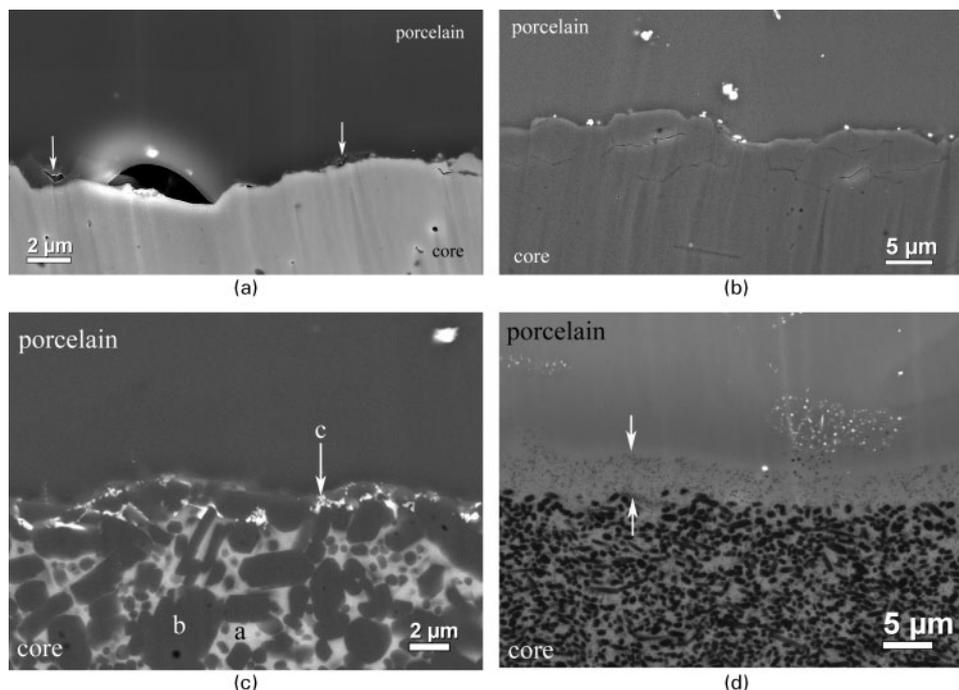
2 Images (SEM) of interface areas of polished cross-sections of bilayered composite samples with core made of *a* zirconia, *b* alumina, *c* glass infiltrated alumina composite and *d* glass ceramics
