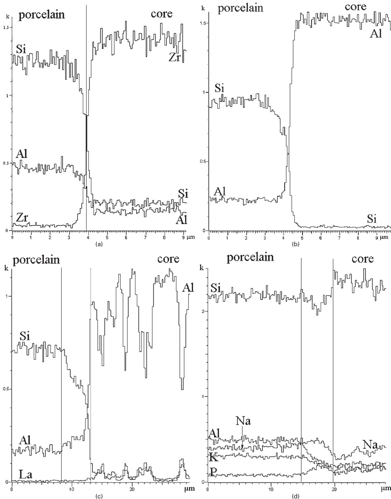
3 Energy dispersive X-ray spectra recorded during linear scanning across interface of bilayer composites with core made of *a* zirconia, *b* alumina, *c* glass infiltrated alumina composite and *d* glass ceramics
