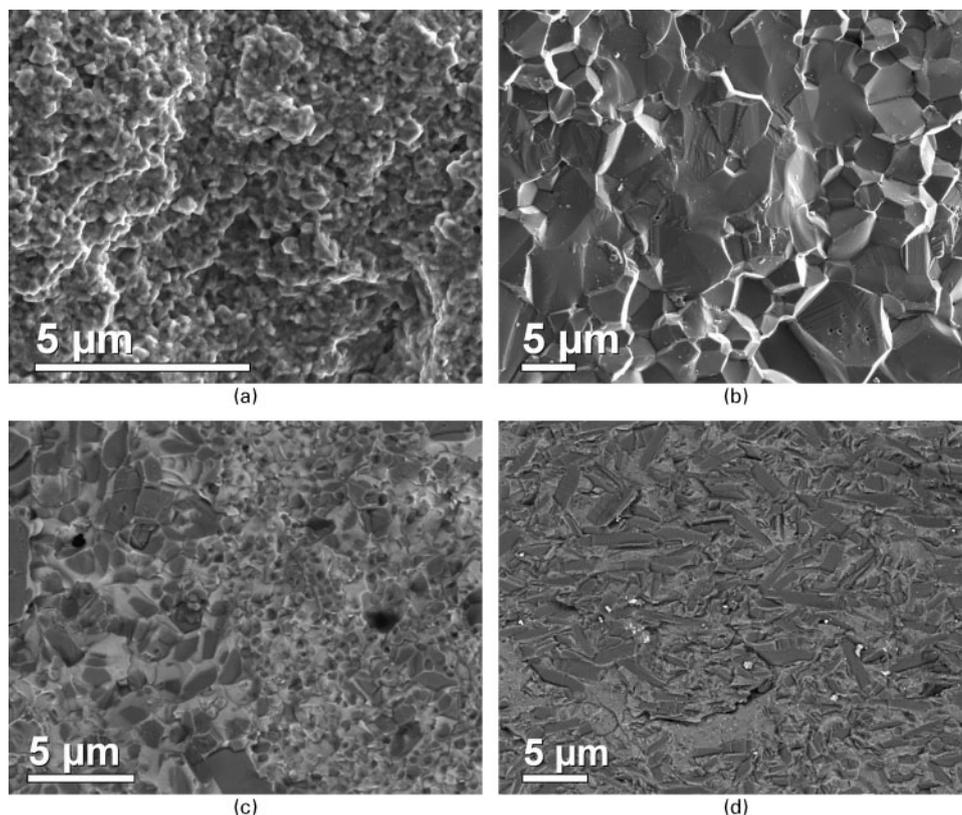
1 Scanning electron microscopy fractography of pure core ceramics of *a* zirconia, *b* alumina, *c* glass infiltrated alumina composite (In-Ceram Al) and *d* glass ceramics (Empress 2)
