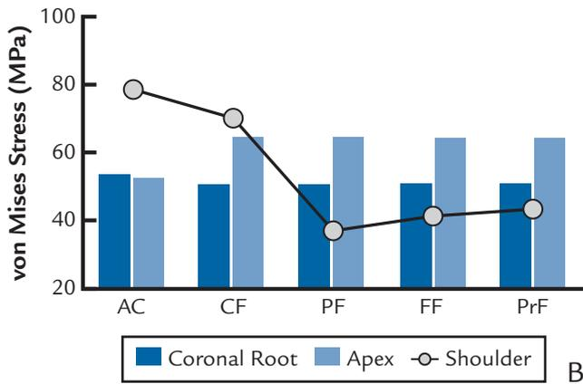
**3** Von Mises stress measured at shoulder, crown, and apex of teeth. A, Gold-alloy-post restored teeth. B, Glass-fiber-post restored teeth.
