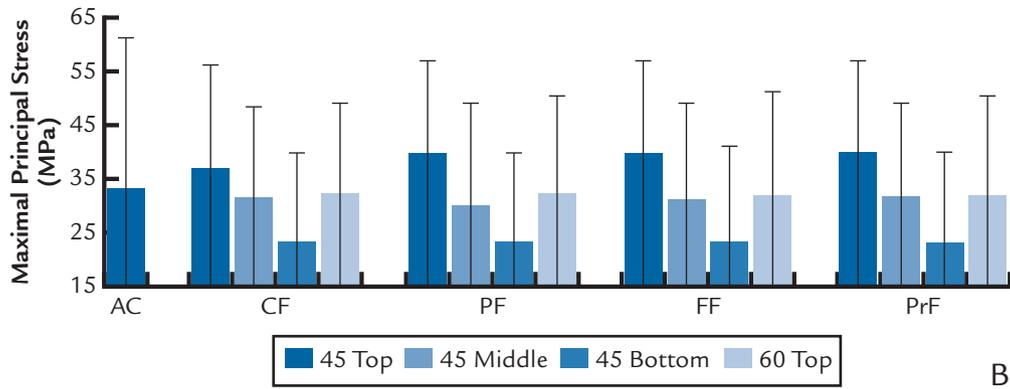
**7** Maximal principal stress (peak and average values) measured at dentin for different loading procedure. A, Gold-alloy-post restored teeth. B, Glass-fiber-post restored teeth.
