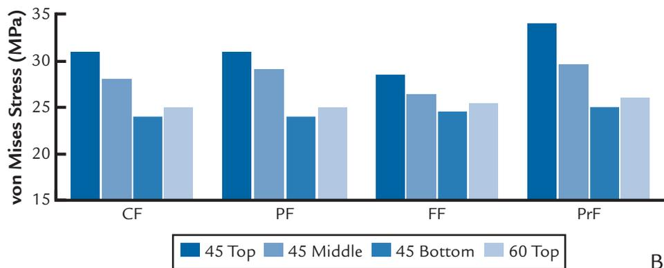
**8** Von Mises stress measured on composite resin and glass-fiber-post under different loading procedures. A, Peak stress measured on composite resin. B, Peak stress measured on glass-fiber-post.
