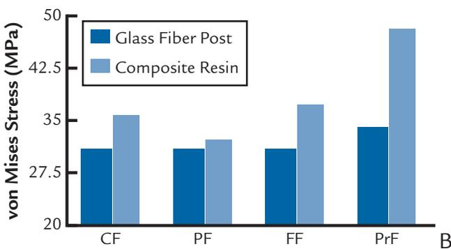
**4** Von Mises stress measured at post and core. A, Gold-alloy-post. B, Glass-fiber-post and composite resin.
