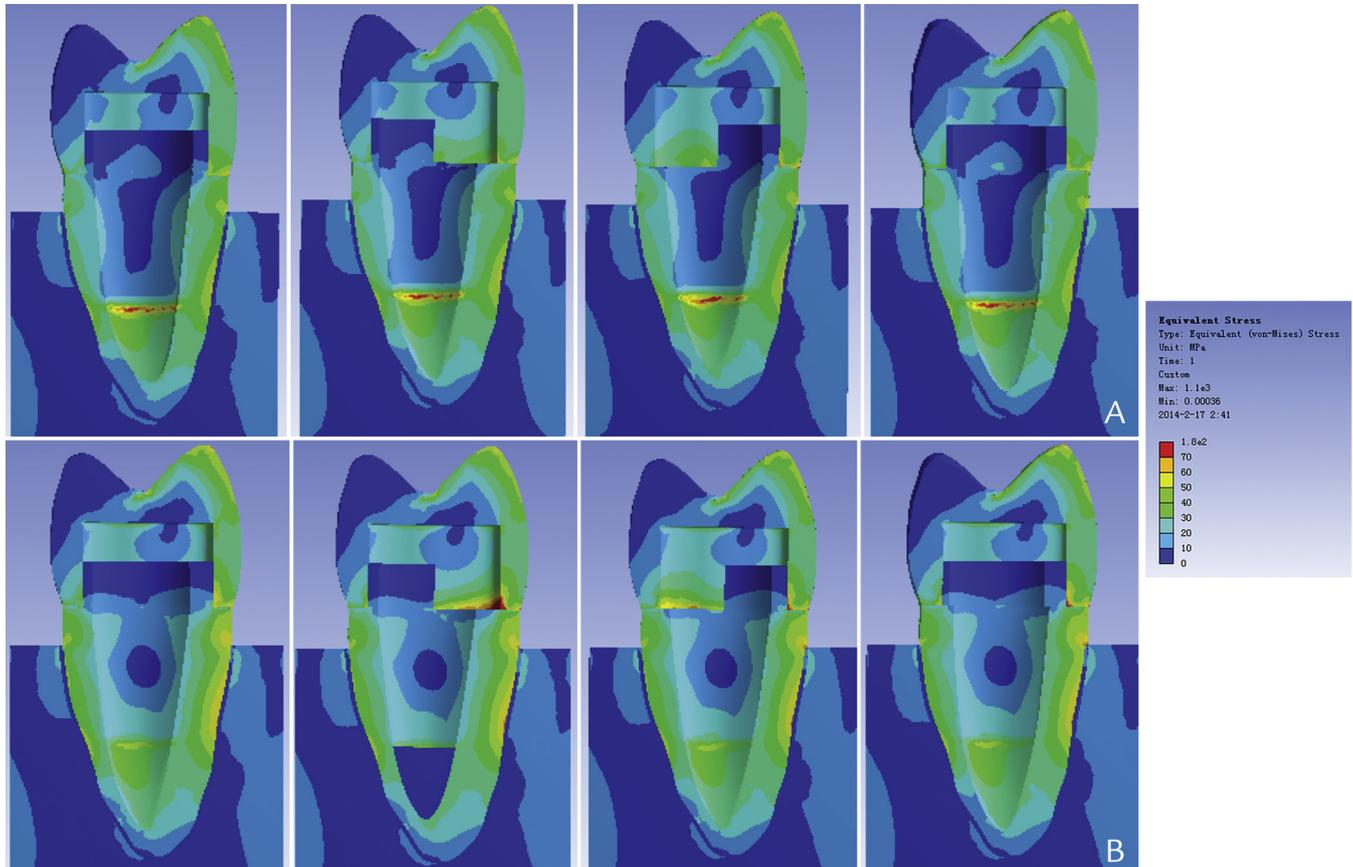
2 Von Mises stress contours of teeth with different ferrules. A, Gold-alloy-post restored teeth. B, Glass-fiber-post restored teeth.
