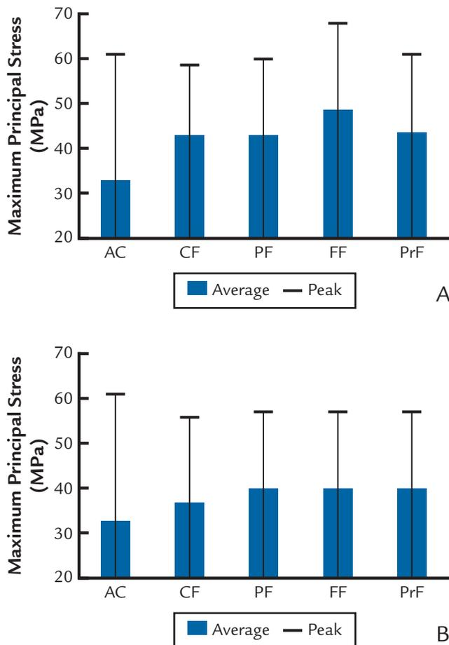
**5** Maximal principal stress measured at dentin. A, Gold-alloy-post restored teeth. B, Glass-fiber-post restored teeth.
