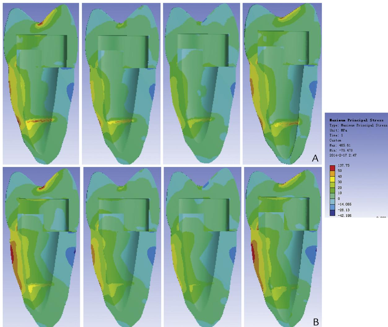
**6** Maximal principal stress contours of palatal ferrule tooth under different loading procedures. A, Gold-alloy-post restored teeth. B, Glass-fiber-post restored teeth. 1. Load on top of 45-degree cusp; 2. Load on middle of 45-degree cusp; 3. Load on bottom of 45-degree cusp; 4. Load on top of 60-degree cusp.
