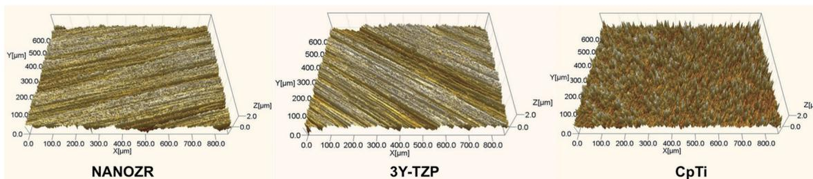
Fig. 1 3D surface topography of NANOZR, 3Y-TZP and CpTi (0.6 mm×0.8 mm) after polishing with 600# abrasive paper.
