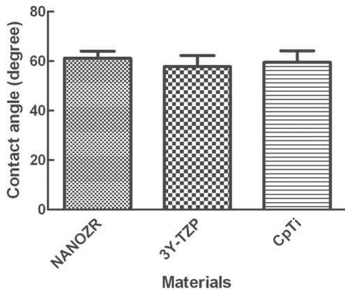
Fig. 5 Contact angle against distilled water of NANOZR, 3Y-TZP and CpTi. There was no significant difference among the three materials ( $p>0.05$ ).
