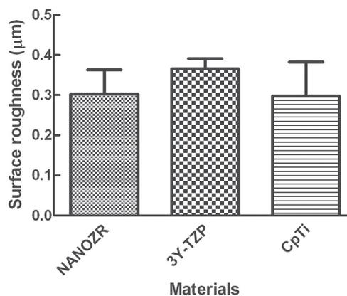
Fig. 2 Surface roughness of NANOZR, 3Y-TZP and CpTi after polishing with 600# abrasive paper. There was no significant difference among the three materials ( $p > 0.05$ ).
