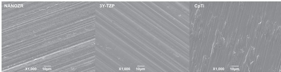
Fig. 3 SEM micrographs of NANOZR, 3Y-TZP and CpTi.
