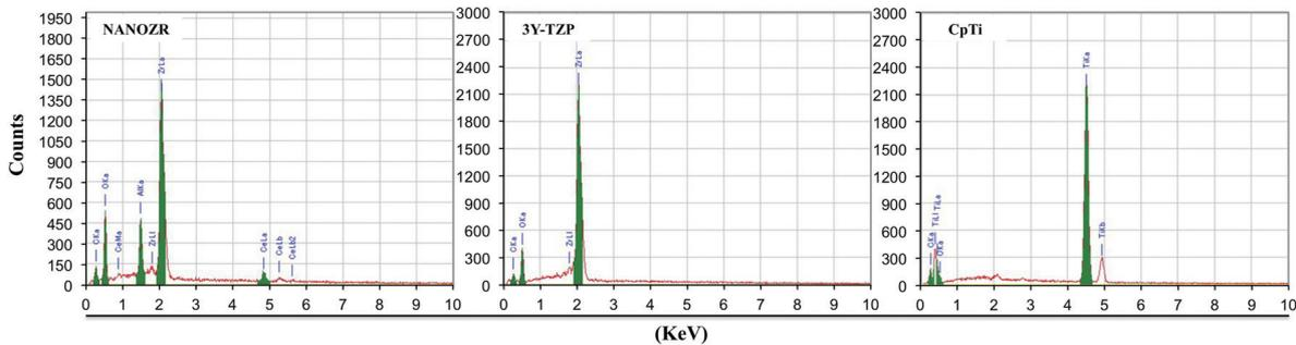
Fig. 4 Surface composition of NANOZR, 3Y-TZP and CpTi.
