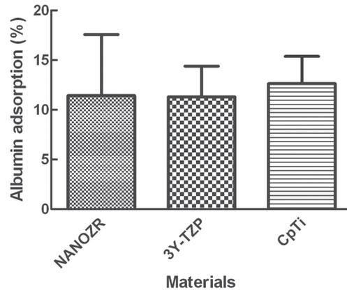
Fig. 6 Bovine serum albumin adsorption rates of NANOZR, 3Y-TZP and CpTi after 1 h incubation. There was no significant difference among the three materials ( $p>0.05$ ).
