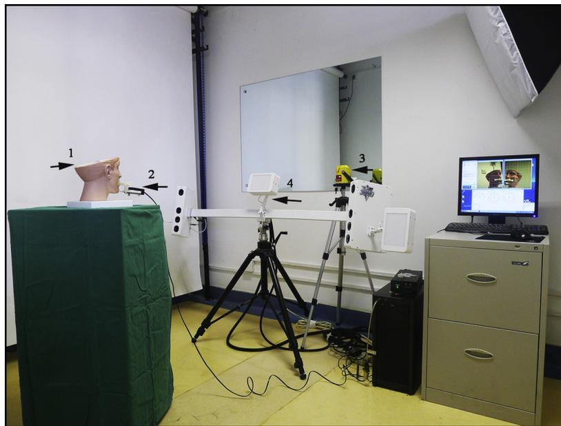
**Fig 2.** Instrument and imaging environment for natural head position recording: 1, physical model; 2, gyroscope; 3, laser collimeter; 4, 3D multicamera system.
