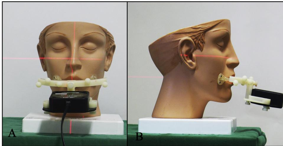
**Fig 1.** Projection of the horizontal laser beam on the physical model. A laser level was used to project a horizontal reference line from ear to ear on a physical model. The orientation was recorded simultaneously by a gyroscope. **A**, frontal view; **B**, lateral view.
