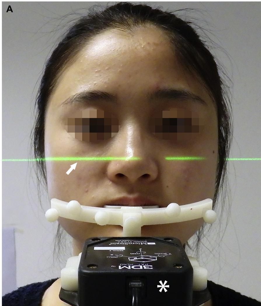
**FIGURE 4.** Recording head positions using the 2 methods. Each test head position was simultaneously recorded by the digital gyroscope (*asterisk*) and by the 3dMDface System and laser level. A, Frontal view show the horizontal laser line (*arrow*) projected on the face and (**Fig 4 continued on next page.**)
