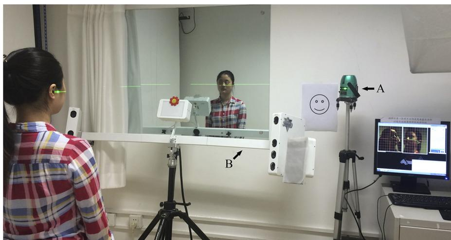
**FIGURE 1.** Setting and instruments used to record head positions. A, Laser level. B, The 3dMDface System. The center flashlight was turned off, and the right and left flashlights were covered with translucent paper to decrease the intensity of the light.
