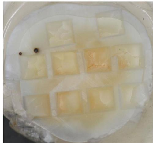
**Fig. 4** Square cavities formed by ablating dentin three-dimensionally, using picosecond laser
