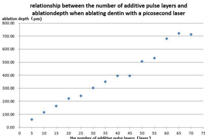
**Fig. 3** Graphic representation of the quantitative relationship between the number of focal plane additive pulse layers and ablation depth during two-dimensional scanning and ablation of dentin using picosecond laser. *Left*, relationship between the number of additive pulse layers and ablation depth when ablating dentin by using a picosecond laser; *y*-axis; *right*,
