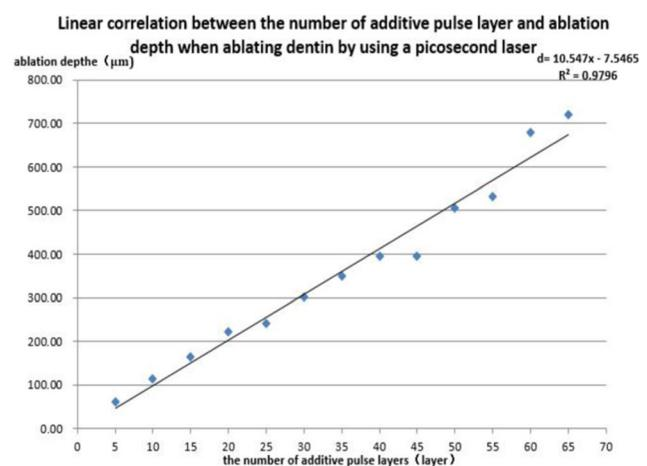
linear correlation between the number of additive pulse layer and ablation depth when ablating dentin by using a picosecond laser. For both panels, the *y*-axis shows ablation depth ( $\mu\text{m}$ ), and the *x*-axis denotes number of pulse layers (layer)
