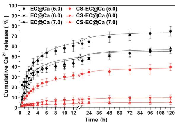
Fig. 5 Cumulative release of  $\text{Ca}^{2+}$  from the  $\text{EC}@\text{Ca}(\text{OH})_2$  and  $\text{CS-EC}@\text{Ca}(\text{OH})_2$  microcapsules was dependent on pH.
