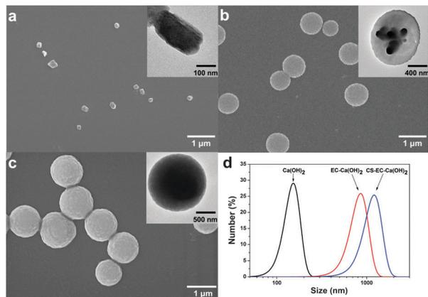
Fig. 1 SEM and TEM (inset) images of three representative samples: (a)  $\text{Ca}(\text{OH})_2$ , (b)  $\text{EC}@\text{Ca}(\text{OH})_2$  microcapsules and (c)  $\text{CS-EC}@\text{Ca}(\text{OH})_2$  microcapsules. (d) Particle size distribution of the samples in water.
