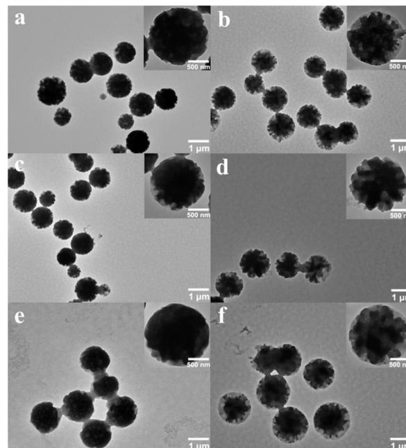
Fig. 6 TEM images of representative microcapsules at low and high (inset) magnifications after release at various pH values and times: (a and b)  $\text{EC}@\text{Ca}(\text{OH})_2$  microcapsules at pH = 7.0 at 0.5 h and 24 h; (c and d)  $\text{EC}@\text{Ca}(\text{OH})_2$  microcapsules at pH = 5.0 at 0.5 h and 24 h; (e and f)  $\text{CS-EC}@\text{Ca}(\text{OH})_2$  microcapsules at pH = 5.0 at 0.5 h and 24 h.
