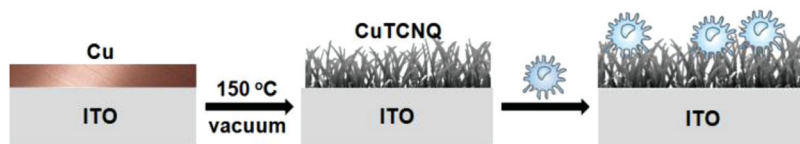
Scheme 1 Schematic illustration of the use of 3D CuTCNQ nanowire biointerfaces for highly efficient cell adhesion.
