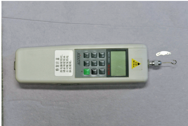
Figure 1. Custom-made contact pressure system with digital force gauge and metal strip.
