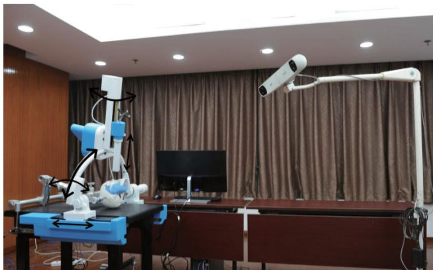
**Fig. 1** The skull phantom and the robot system setup with five degrees of freedom (black arrows).
