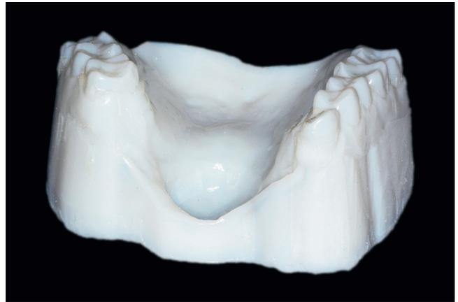
**Figure 6.** Resin cast fabricated with rapid prototyping (3D printing).
