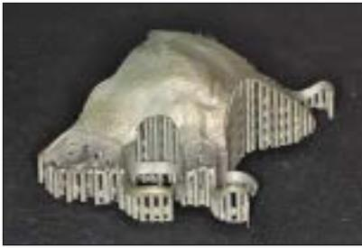
**Fig 4** Cobalt-chromium alloy framework directly fabricated using the rapid prototyping system.
