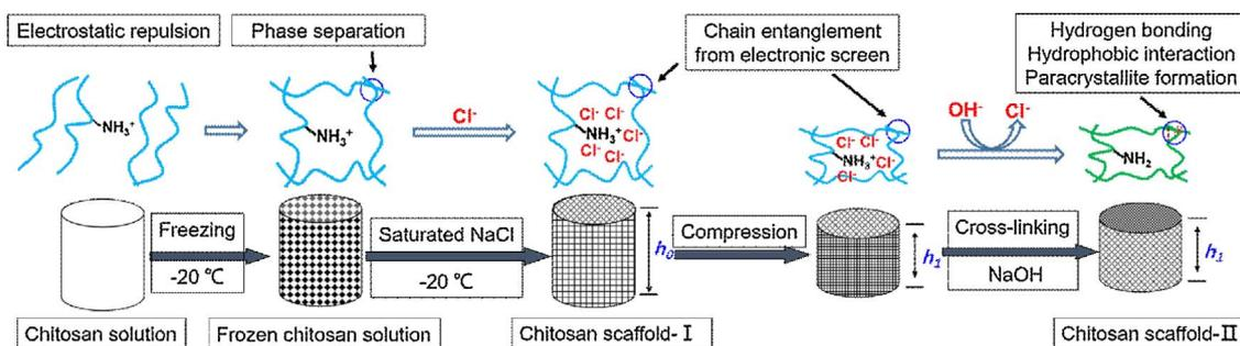
Scheme 1. Schematic illustration of the process and mechanism for fabrication of chitosan scaffolds.
