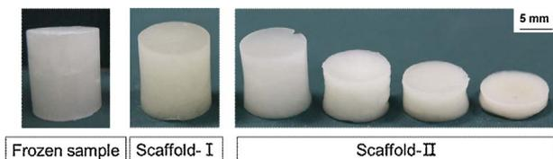
Fig. 1. Digital images showing the morphologies of frozen chitosan solution, chitosan scaffold-I, and scaffold-II.
