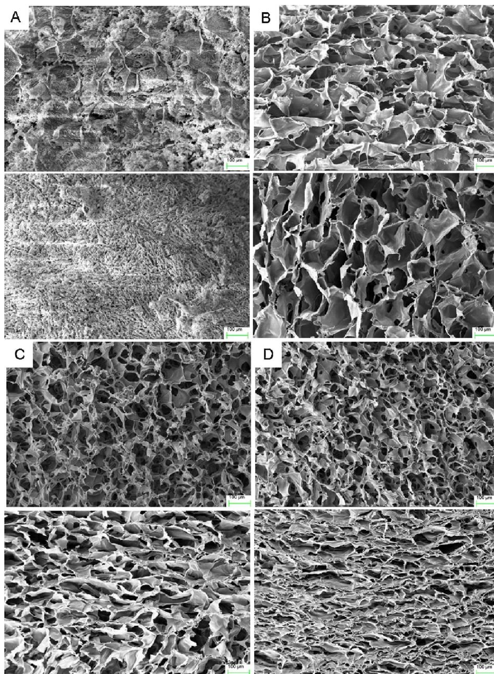
Fig. 2. SEM images of the scaffolds: (A) scaffold-I at 20 mg/ml; scaffold-II at different compressive ratios ( $R$ ) (B)  $R = 1$ , (C)  $R = 3$ , (D)  $R = 6$ . Top: Section perpendicular to compression direction; Bottom: Section parallel to compression direction.
