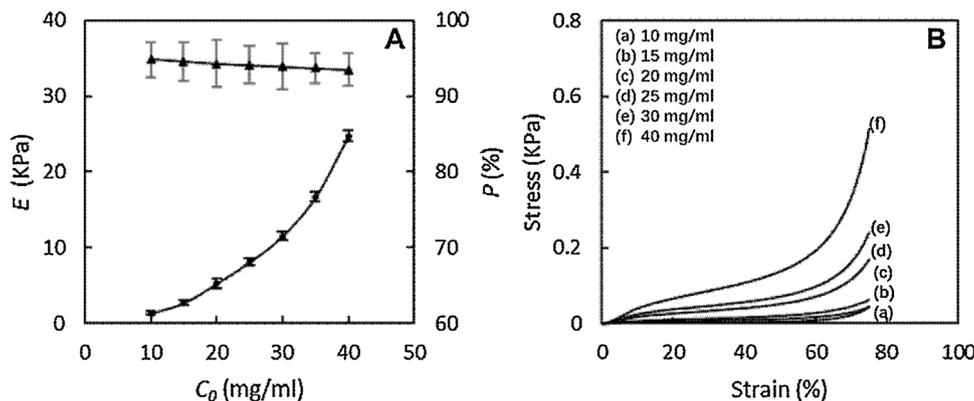
Fig. 6. The properties of scaffold-II at different initial concentrations ( $C_0$ ): (A) compressive elastic modulus ( $E$ ) and porosity ( $P$ ); (B) compressive stress-strain curve.
