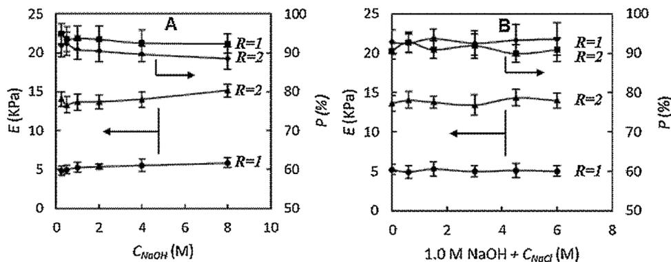
Fig. 5. The effects of  $C_{NaOH}$  on the compressive elastic modulus ( $E$ ) and porosity ( $P$ ) of scaffold-II: (a)  $R = 1$  and (b)  $R = 2$ .
