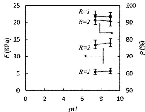
Fig. 7. pH-responsive properties, compressive elastic modulus ( $E$ ) and porosity ( $P$ ), of scaffold-II with  $R = 1$  and  $R = 2$  in  $1 \times$  PBS ( $pH = 3.0, 5.0, 7.4$  and  $9.0$ ).
