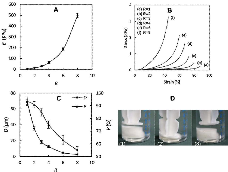
Fig. 4. The properties of scaffold-II at different compressive ratios ( $R$ ): (A) compressive elastic modulus ( $E$ ); (B) compressive stress–strain curve; (C) average pore diameter ( $D$ ) and porosity ( $P$ ); (D) shape recovery of sample in  $1 \times$  PBS (pH = 7.4) at  $R = 2$ .
