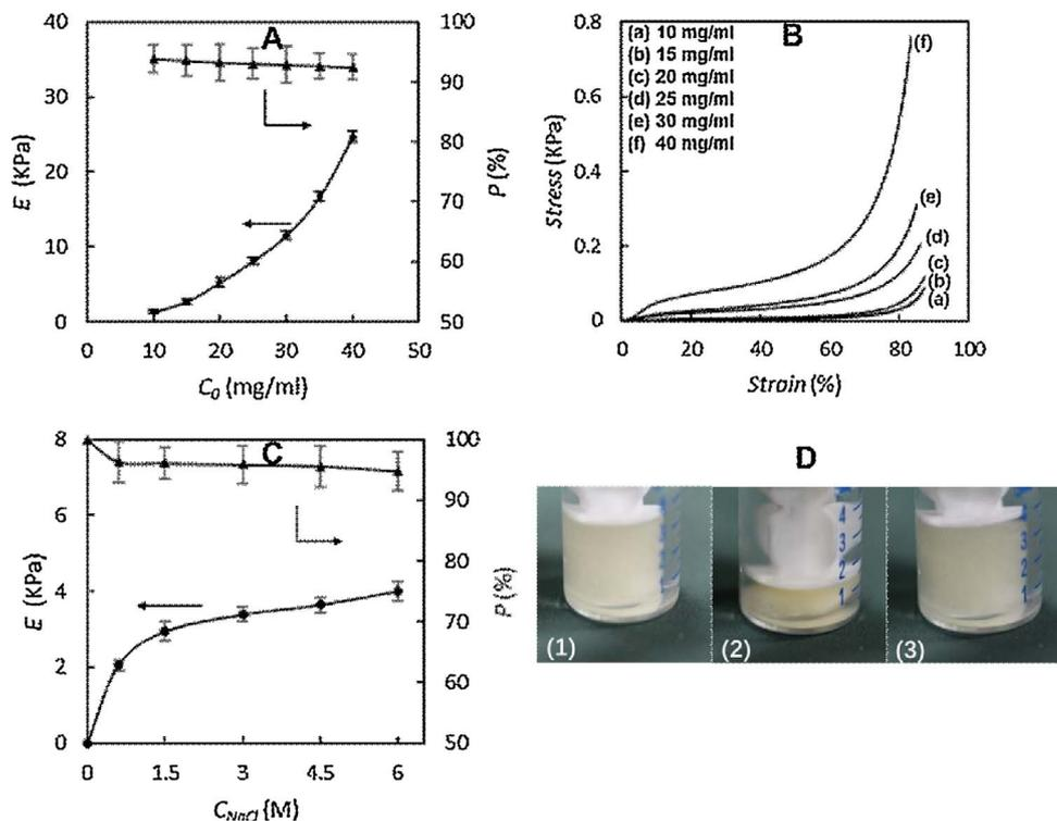
Fig. 3. The properties of scaffold-I. (1) Different original chitosan concentration ( $C_0$ ): (A) compressive elastic modulus ( $E$ ) and porosity ( $P$ ), (B) compressive stress–strain curve and (2)  $C_0 = 20$  mg/ml: (C)  $E$  and  $P$  with different NaCl solutions ( $C_{NaCl}$ ), (D) shape recovery in NaCl solution ( $C_{NaCl} = 3$  M).
