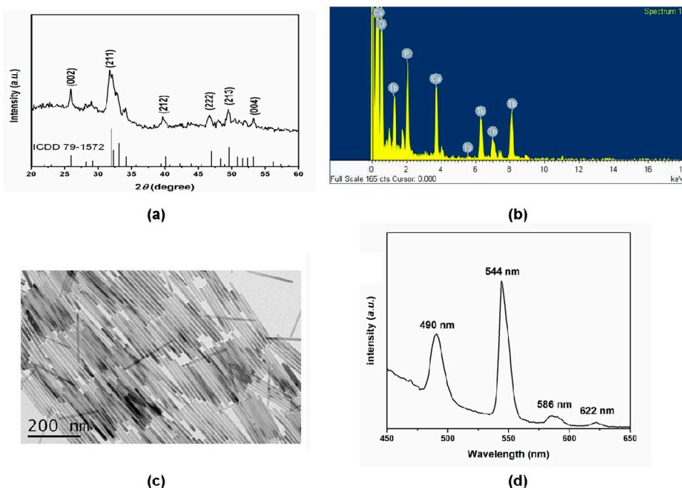
**Figure 1.** Characterization of  $\text{Tb}^{3+}$ -doped hydroxyapatite (HA-Tb) nanorods: (a) X-ray diffraction pattern of HA-Tb nanorods after hydrothermal synthesis; (b) elemental mapping of HA-Tb nanorods by transmission electron microscopy (TEM) with energy-dispersive spectroscopy; (c) representative TEM image showing the nanorod morphology; and (d) luminescence spectrum of HA-Tb crystals.
