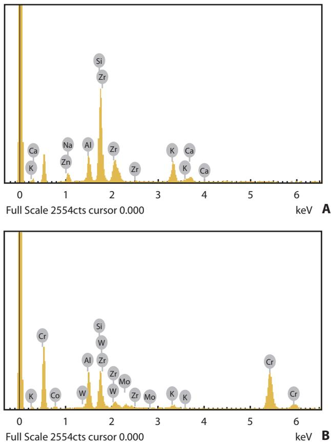
**Figure 4.** Representative spot EDS scanning spectrum of the arrows “a” and “b” in Figure 3. A, “a”. B, “b”. EDS, energy-dispersive x-ray spectroscopy.
