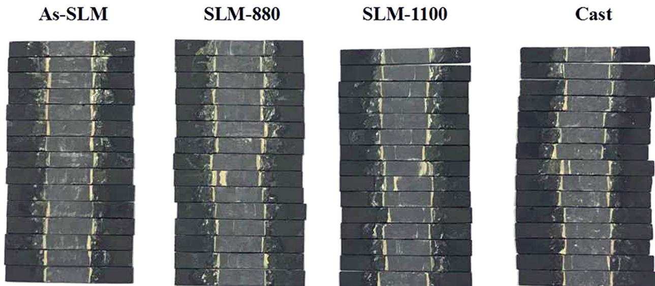
**Figure 2.** Digital image of specimen surfaces after fracture failures. As-SLM, not subjected to heat treatment. SLM-880, heat treatments at 880°C. SLM-1100, heat treatment at 1100°C.
