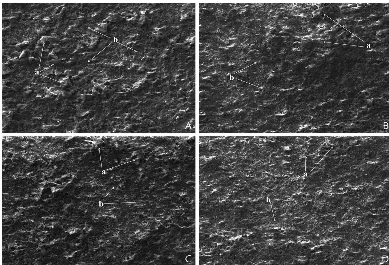
**Figure 3.** Scanning electron micrographs of fractured metal surfaces. A, As-SLM. B, SLM-880. C, SLM-1100. D, cast. (20.0 kV, original magnification  $\times 250$ ). Arrows labeled "a" and "b" indicate representative spot EDS scanning spectrum in Figure 4. As-SLM, not subjected to heat treatment. EDS, energy-dispersive x-ray spectroscopy. SLM-880, heat treatments at 880°C. SLM-1100, heat treatment at 1100°C.
