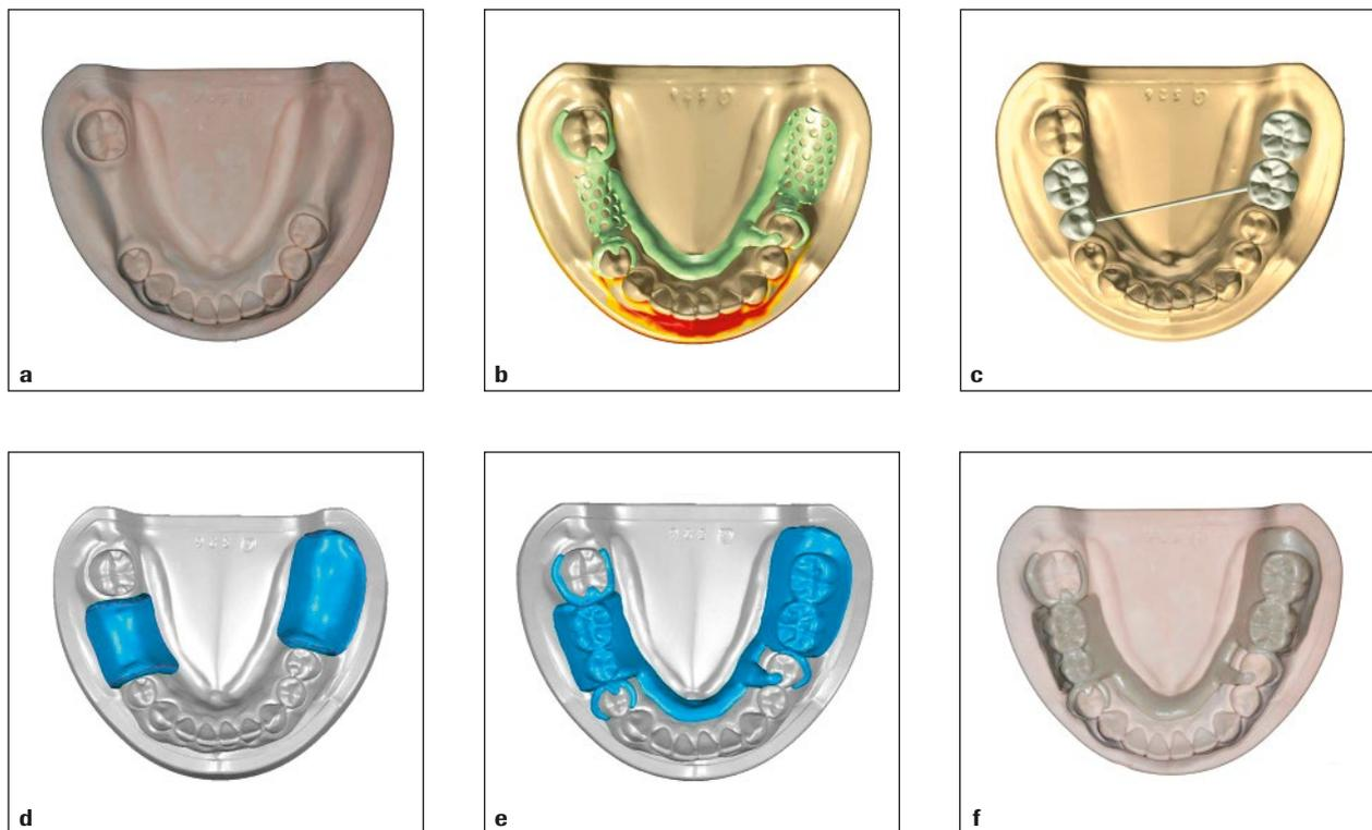
**Fig 1** Computer-aided design/computer-aided manufacture (CAD/CAM) process for one-piece polyetheretherketone (PEEK) removable partial denture (RPD). **(a)** Standard stone cast of partially edentulous mandible. **(b)** Framework designed in Dental System. **(c)** Arrangement of artificial teeth in Dental System. **(d)** Denture base created in Geomagic Studio. **(e)** Digitally designed RPD. **(f)** One-piece PEEK RPD was well-seated on the stone cast.
