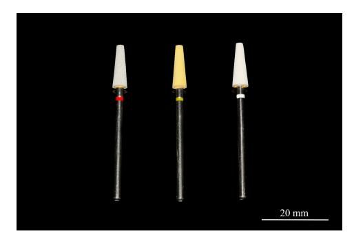
Figure 3. Rubber diamond polishers used in this study. Coarse grit (grey; left), medium grit (yellow; middle), and fine grit (white; right) polishers.
