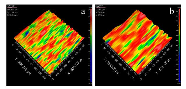
Figure 6. Surface area roughness (Sa) of CZ and SGZ specimens characterized by the white light interferometer. (a) Surface of CZ after polishing; (b) Surface of SGZ after polishing.
