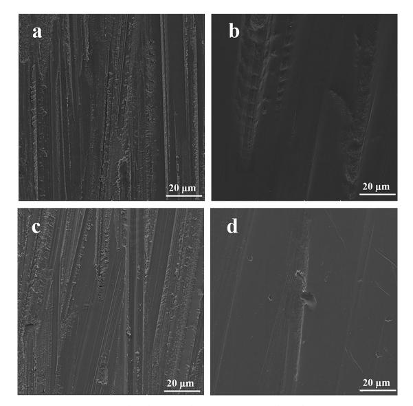
Figure 8. SEM images taken on the surface of the two different zirconia ceramics after surface treatment. (a) CZ specimen after grinding; (b) CZ specimen after polishing; (c) SGZ specimen after grinding; (d)SGZ specimen after polishing.
