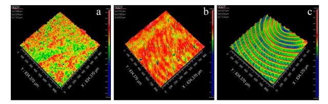
**Figure 4.** Surface area roughness (Sa) of CZ and SGZ specimens characterized by the white light interferometer. (a) Blank-machined surface of CZ before grinding procedure; (b) Surface of SGZ performed by 3D gel deposition process before grinding; (c) Green-machined internal surface of SGZ before grinding.
