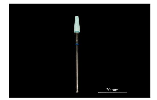
Figure 2. Ceramic diamond grinders used in this study.
