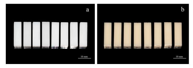
Figure 1. Two types of bar-shaped dental zirconia specimens. (a) SGZ specimens; (b) CZ specimens.
