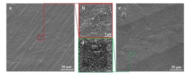
Figure 7. SEM images taken on the surface of the as prepared specimens. (a-b) Blank-machined surface of CZ; (c-d) Surface of SGZ prepared by 3D gel deposition.
