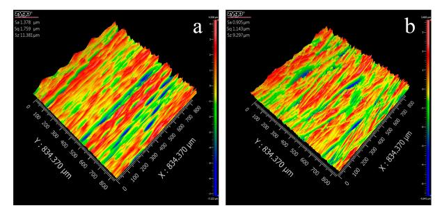
Figure 5. Surface area roughness (Sa) of CZ and SGZ specimens characterized by the white light interferometer. (a) Surface of CZ after grinding; (b) Surface of SGZ after grinding.
