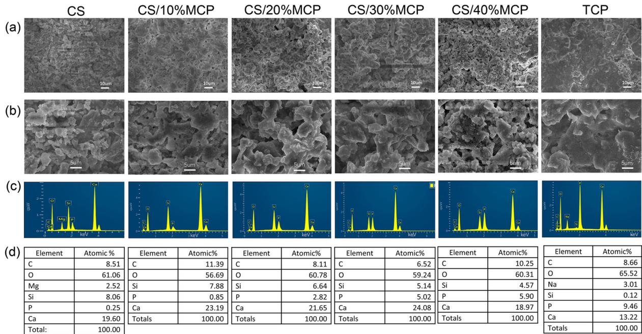
**Figure 1.** Morphochemical characterization of cement. (a), (b) SEM view of the cements surface, magnified 1000 times and 3000 times respectively. (c) EDX spectra of the whole area. (d) The elemental X-ray microanalysis performed on the cement surface.
