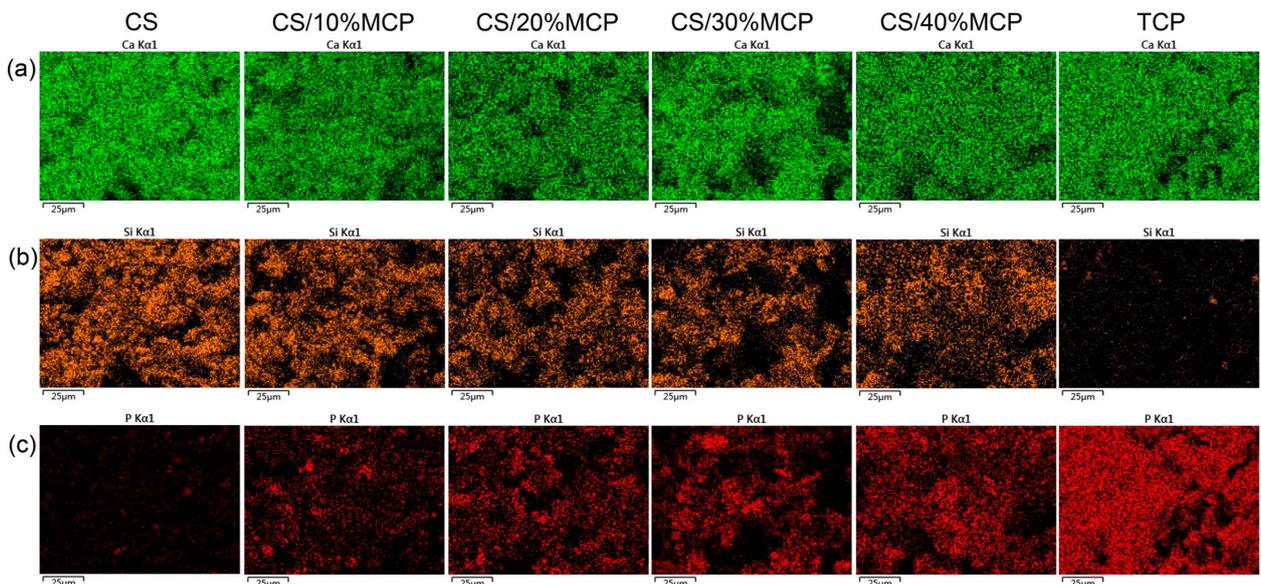
**Figure 2.** SEM-EDS elemental maps for (a) Ca, (b) Si and (c) P (magnified 1000 times) showed that with increasing MCP content, the content of Si decreased, the content of P increased and the content of Ca basically remained unchanged.
