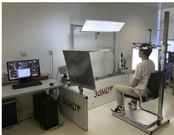
**FIGURE 1.** The 3dMD-Face Dynamic System (3Q Technologies, Atlanta, GA) and the fixing head frame.
