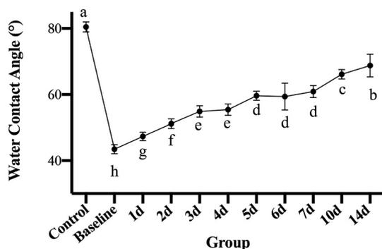
Fig. 7. Water contact angles at the zirconia surface over time. (Values indicated by the same lowercase letters are not significantly different) ( $p > 0.05$ ).
