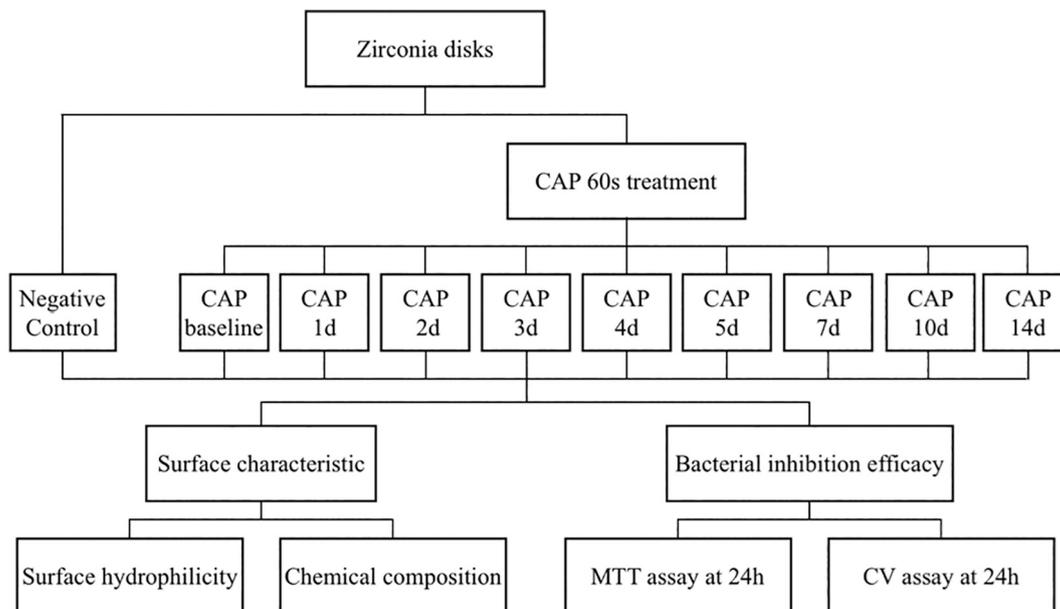
**Scheme 2.** Flowchart of the evaluation of time-dependent change of CAP-treated zirconia.
