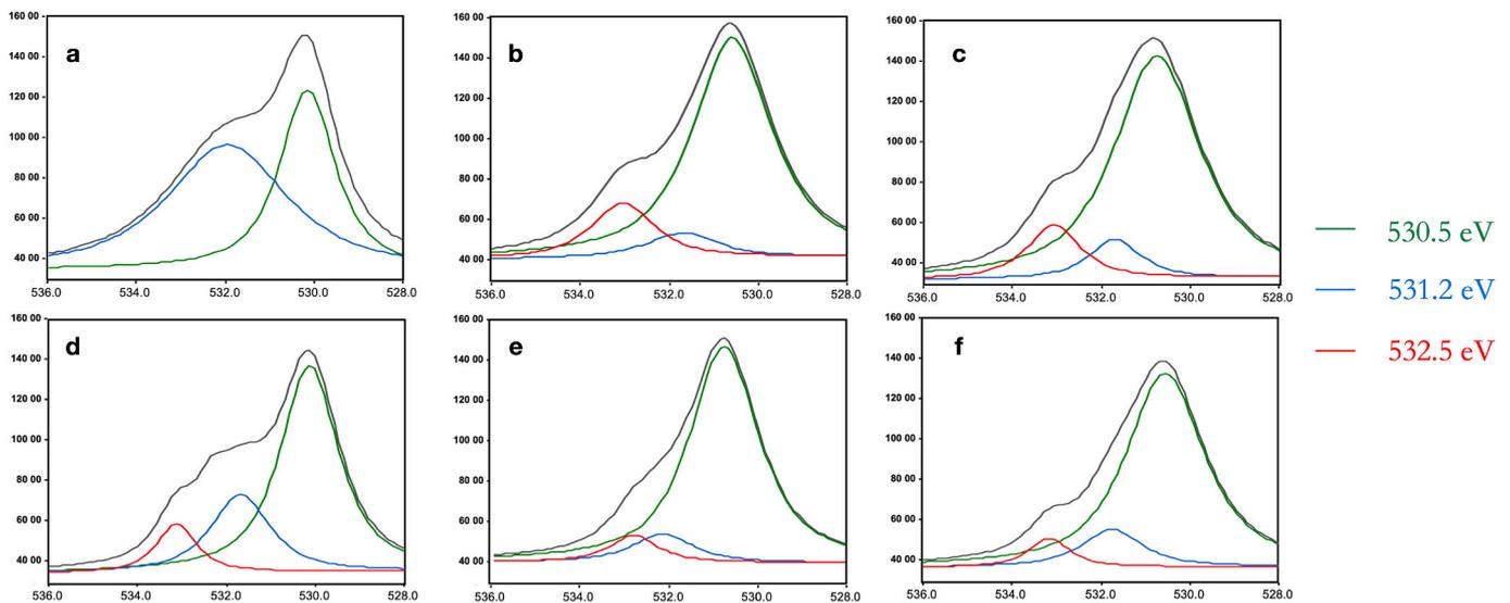
Fig. 8. XPS O1s high-resolution image of the negative control (a), CAP baseline (b), CAP 1d (c), CAP 5d (d), CAP 10d (e), and CAP 14d (f). X axis: Binding energy, Y axis: Counts.
