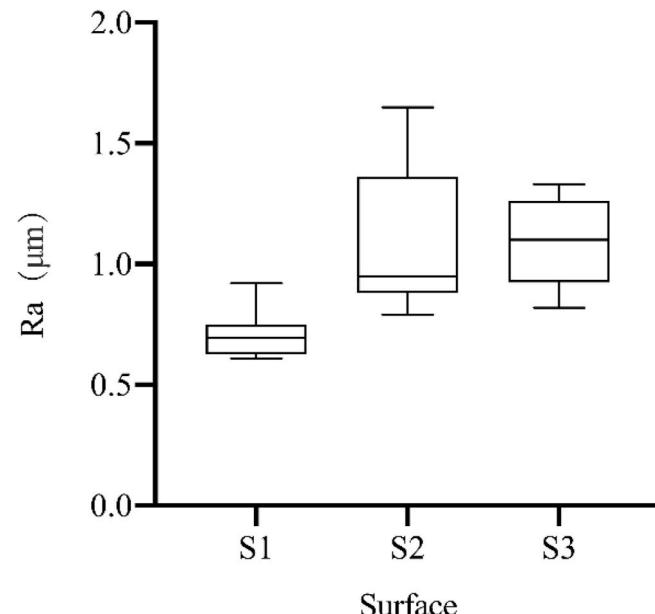
Fig. 6. Box plots of the roughness of surfaces S1, S2 and S3.
