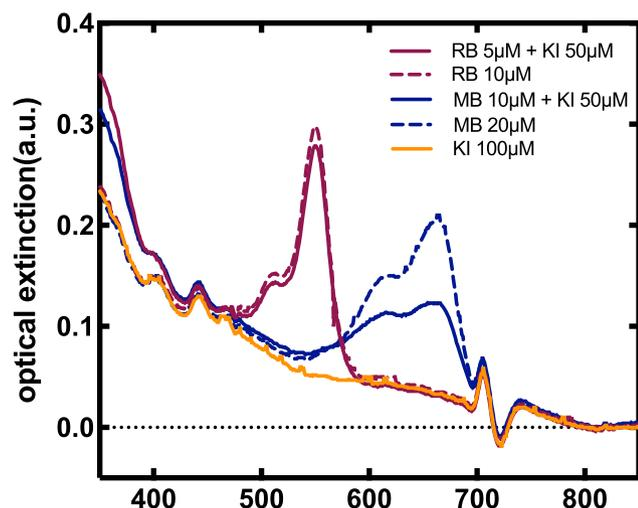
Fig. 1. The absorption spectrum of methylene blue (MB) and rose bengal (RB) with or without potassium iodide (KI) with peak absorptions around 660 and 550 nm, respectively.
