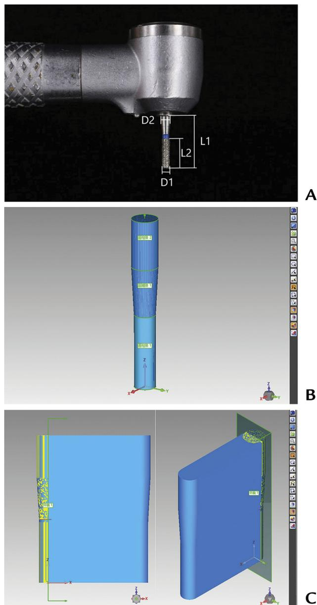
**Figure 3.** A, Parameter measurement of diamond rotary instrument. B, Three-dimensional modeling of diamond rotary instrument. C, Three-dimensional modeling of movement path of diamond rotary instrument.
