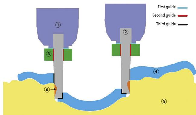
**Figure 10.** Triple guiding mechanism of template. ① Handpiece. ② Straight flat end diamond rotary instrument. ③ Handpiece guide rail. ④ Retainer of template. ⑤ Cast of partially edentulous mandible. ⑥ Virtual preparation of abutment teeth.
