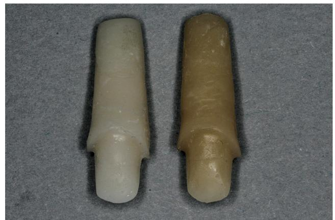
**Figure 2.** Shade A1 and A3 abutment specimens.
