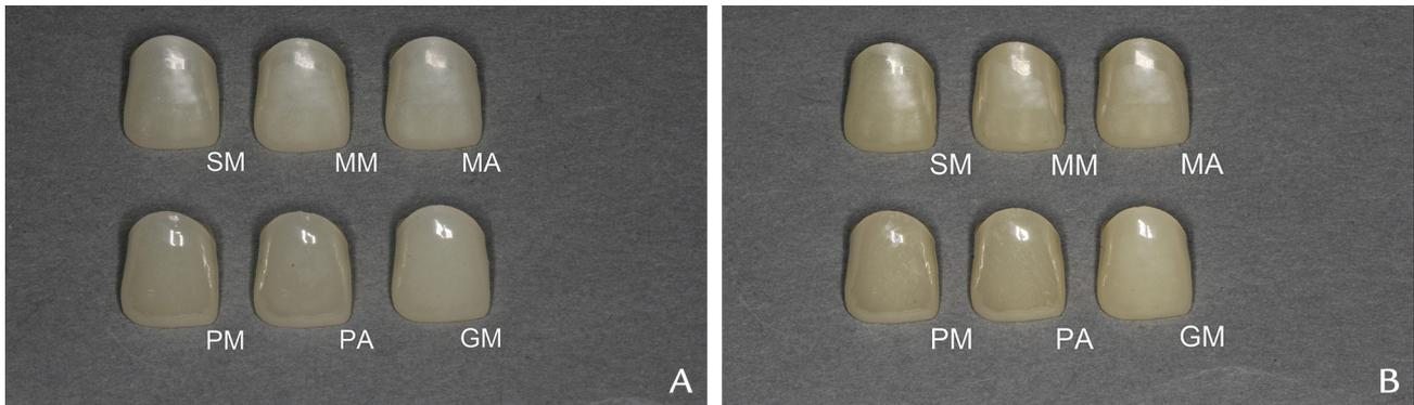
**Figure 1.** Six groups of self-glazed zirconia crowns of each shade. A, Shade A1. B, Shade A3. GM, glazed/milled; MA, milled/airborne-particle abraded; MM, milled/milled; PA, polished/airborne-particle abraded; PM, polished/milled; SM, self-glazed/milled.
