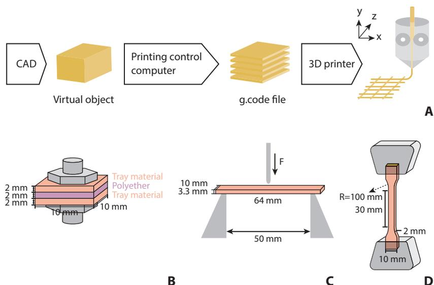
**Figure 1.** Study overview. A, Process flow of 3D printing technology: coordinate axes in accordance with printing orientation used. B, Tensile bond strength test. C, Three-point bend test. D, Tensile test. CAD, computer-aided design.
