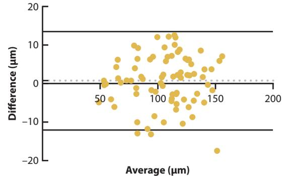
**Figure 5.** Bland-Altman plots of difference (triple scan minus silicone replica) against average of cement-gap thickness measured by triple-scan method and by silicone replica method. 95% limits of agreement shown by solid lines. Bias shown by dashed line.
