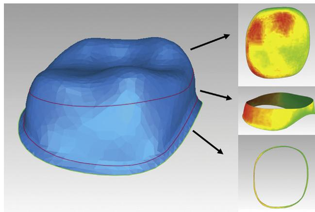
**Figure 3.** Three areas (occlusal, axial, marginal) defined for analysis by “3D Compare” and representative color-coded difference images showing 3D cement-gap thickness. *Red* indicates large thickness and *green* indicates small thickness.
