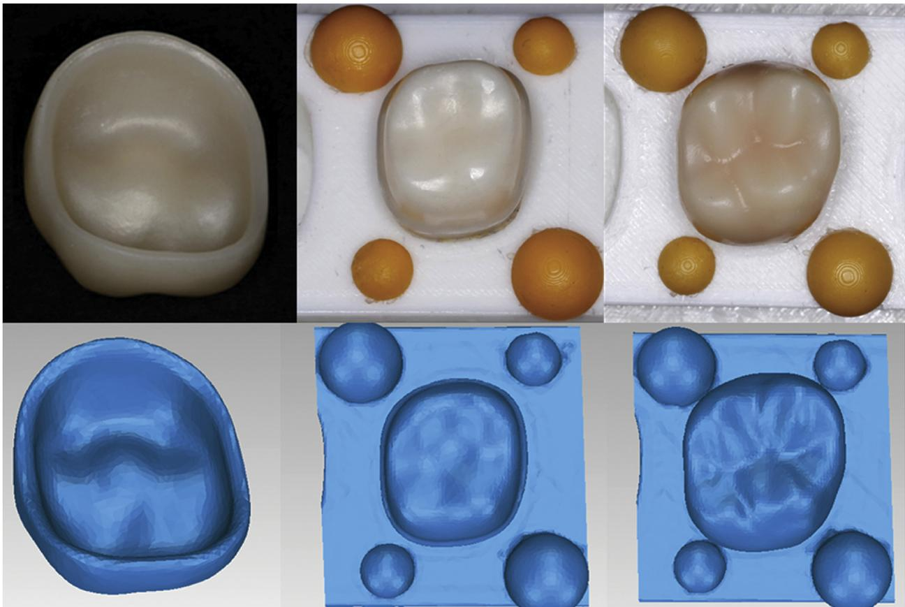
**Figure 1.** Specimens and scan data sets in triple-scan method. Left to right: crown, abutment fixed in base, crown seated on abutment.
