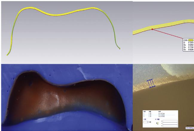
**Figure 4.** Corresponding cross-section and measurement of cement gap in triple-scan method and in physical silicone replica.
