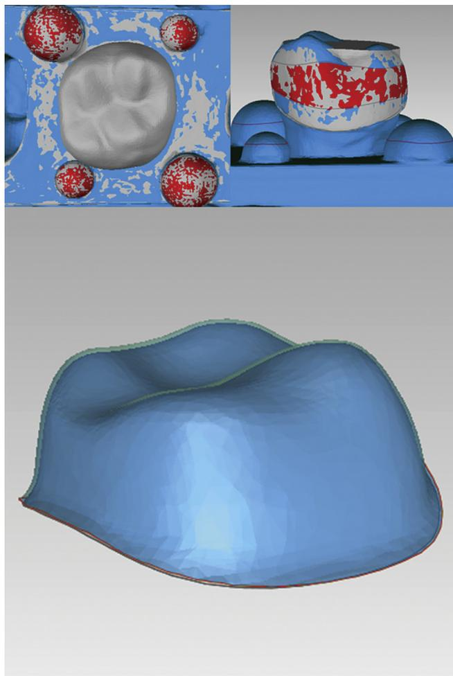
**Figure 2.** With data seated aligned to data abutment and data crown aligned to data seated, cement-gap between intaglio surface and abutment surface was obtained. Common area chosen for alignment shows interweaving surfaces (*red and gray*)
