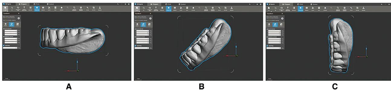
**Figure 2** Printing configuration of the mandibular complete denture in the software in 3 different build orientations. (A) 0 degrees. (B) 45 degrees. (C) 90 degrees.
