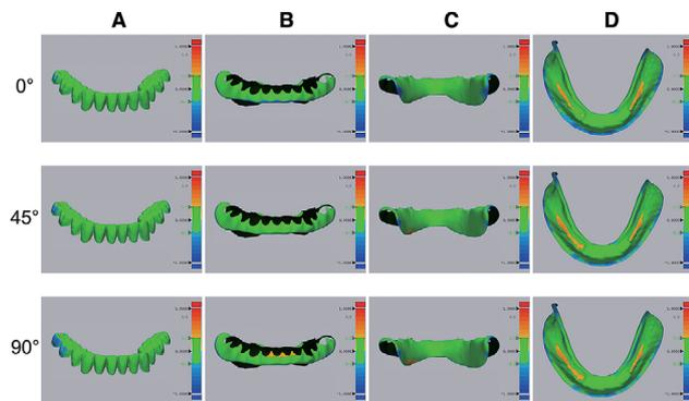
**Figure 4** Representative surface-matching color maps from 3 build orientations (0°, 45°, 90°). Green areas indicate dimensional difference within 0.03mm, blue areas indicate negative discrepancies, yellow and red areas indicate positive discrepancies. (A) Teeth surface. (B) Denture extension surface front view. (C) Denture extension surface back view. (D) Intaglio surface.
