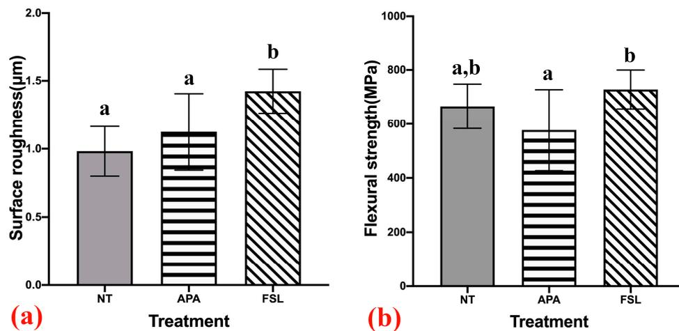
**Figure 3.** (a) The mean surface roughness values ( $R_a$ ), where the  $R_a$  value for the FSL group was significantly the highest ( $p < 0.05$ ); (b) the mean flexural strength values ( $p < 0.05$ ), where the result in the FSL group was significantly higher than that in the APA group ( $p < 0.05$ ). NT: no treatment group; APA: airborne particle abrasion group; FSL: femtosecond laser group.
