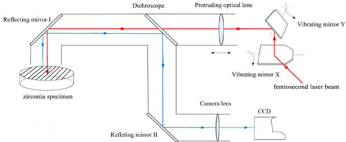
**Figure 1.** Schematic of the FSL surface treatment system and laser trajectory during surface treatment of the specimen. The red line indicates the propagation path of the FSL in the system, and the blue line indicates the light from the surface treatment result received by the charge-coupled device, which monitored the real-time processing results as the laser processed the specimen surface.
