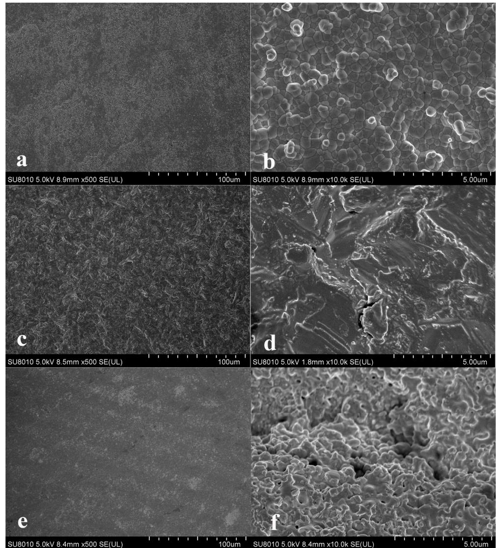
**Figure 2.** SEM images of zirconia surfaces from different groups at 500 $\times$  and 10,000 $\times$  magnifications: (a,b) NT; (c,d) APA; and (e,f) FSL. NT: no treatment group; APA: airborne particle abrasion group; FSL: femtosecond laser group.
