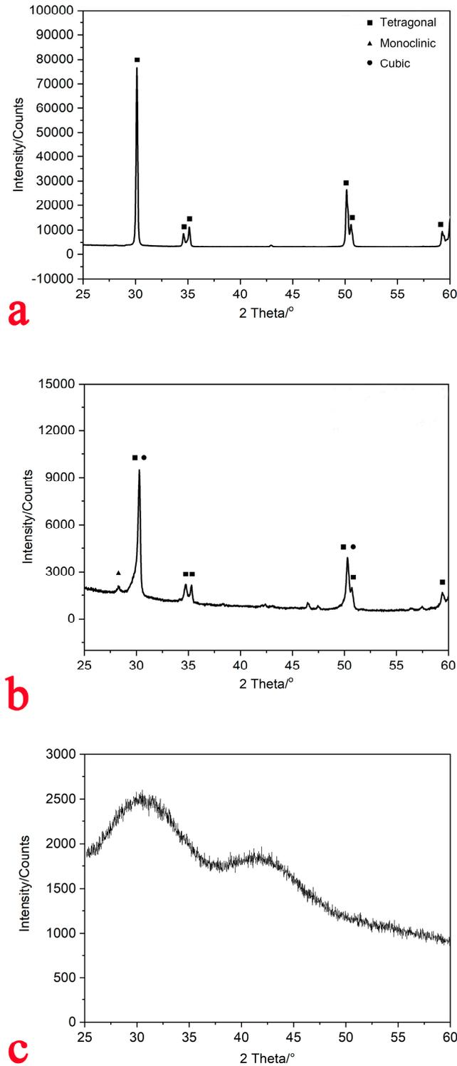
**Figure 4.** XRD images of zirconia surface from different groups: (a) For NT (no treatment group), the zirconia surface for NT was completely tetragonal-phase; (b) for APA (airborne particle abrasion group), the tetragonal phase ratio of the surface was low, with a small amount of monoclinic and cubic phases; and (c) for FSL (femtosecond laser group), there may be an amorphous phase, as it was also possible to form salt crystals on zirconia surfaces treated with FSL.
