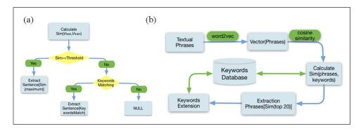
**Figure 2.** (a) Hybrid method of attribute recognition. Principles of attribute selection are described, using keyword-based and deep learning methods, and (b) workflow of attribute values recognition. Deep learning methodology was applied to generate new keywords to expand the keywords database.
