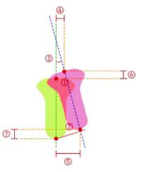
**FIGURE 5** The measurement methods of the deviations between the planed and inserted implants. 1 entry deviation (3D deviation in the coronal aspect of the alveolar ridge); 2 apex deviation (3D deviation in the apical area of the implant); 3 angular deviation; 4 entry horizontal deviation; 5 apex horizontal deviation; 6 entry depth deviation; and 7 apex depth deviation
