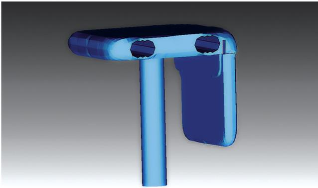
**Figure 1.** Predesign of film holder with 2 perpendicular plates (occlusal plate and imaging plate), guide post, and clip.
